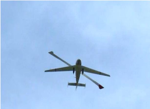
*CarterCopter PAV flyover at 112 rotor rpm.*
