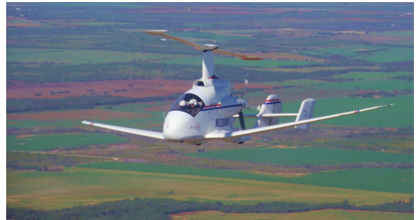
CarterCopter Four-place Personal Air Vehicle (PAV) achieved 214 mph true airspeed at 18,000 ft.
